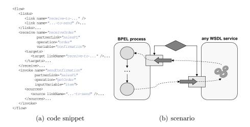
Figure 4: Invocation of a long-running BPEL process
