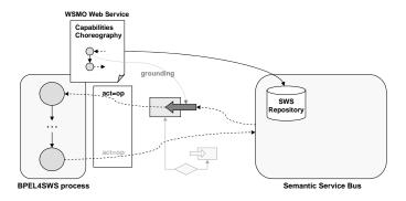
Figure 9: Discovery and invocation of a long-running BPEL4SWS process based on a WSMO WS description.
