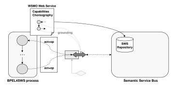
Figure 7: Discovery and invocation of a short-running BPEL4SWS process based on a WSMO WS description.
