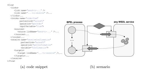
Figure 5: Non-blocking invocation of a WSDL service
