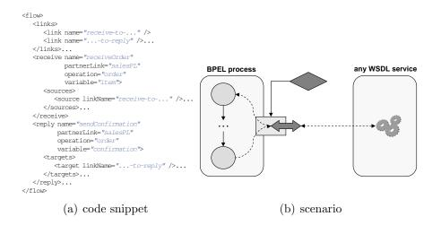
Figure 2: Invocation of a short-running BPEL process
