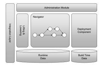
Figure 11: Architecture of a BPEL4SWS Engine.
